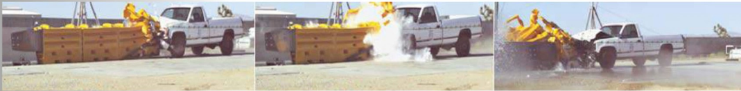
SLED™ TL-3 4500 lb. Pick-Up Truck Impact Attached to Concrete Median Barrier Wall
