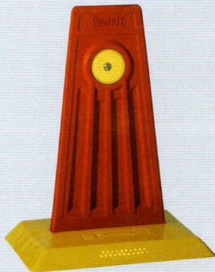
Art. 5062 two-way reflective Dimensions: 220 x 150 x 285 mm Base plate 25 mm high with 2 x 21 glass elements, rubber flag with reflective sheeting
