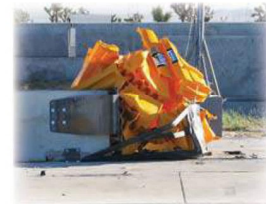
Inline TL-3 Truck Test Post Impact
