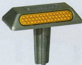
Art. 5201 one-way reflective Art. 5202 two-way reflective Dimensions: 100 x 50 x 20 mm Length anchoring shank: 60.4 mm Aluminium body with 1 or 2 x 43 glass elements, 19° tilted
