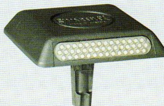
Art. 3547 one-way reflective Art. 3548 two-way reflective Dimensions: 100 x 100 x 19.8 mm Length anchoring shank: 50 mm Aluminium body with 1 or 2 x 43 glass elements, 19° tilted
