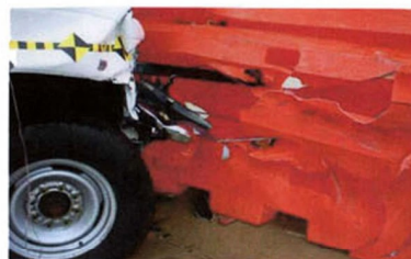
Sentry Water-Cable Barrier™ after a 25° entrance angle impact
