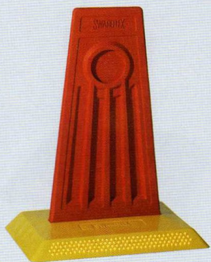
Art. 5017 one-way reflective Art. 5018 two-way reflective Dimensions: 220 x 150 x 285 mm Base plate 25 mm high with 1 or 2 x 128 glass elements, rubber flag without reflector
