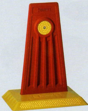
Art. 5020 two-way reflective Dimensions: 220 x 150 x 285 mm Base plate 25 mm high with 1 or 2 x 128 glass elements, rubber flag with 2 round glass reflectors
