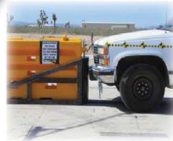
Inline TL-3 Truck Test Pre Impact
