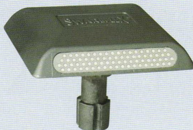
Art. 5031 one-way reflective Art. 5032 two-way reflective Dimensions: 149 x 149 x 27 mm Length anchoring shank: 80 mm Aluminium body with 1 or 2 x 76 glass elements (also available with 1 or 2 x 39 glass elements).
