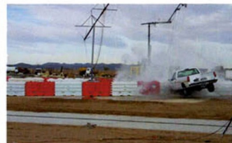
4,409lb (2,000kg) pick-up truck at 25° Impact Angle at 45mph (70kph)
